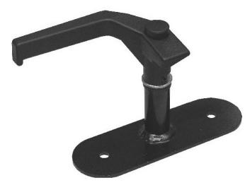
This easy to operate window handle is designed to fit comfortably in the hand for top and side hinged windows for on and offhighway vehicles. Featuring 90 degree rotation with steel mounting plate and glass filled nylon handle.
